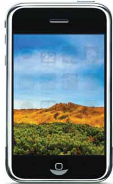
Visible image sticking with conventional amorphous silicon AMOLED
