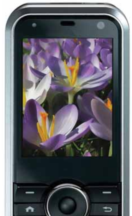
Polysilicon AMOLED with IGNIS AdMo-p™ technology (mura-free)
