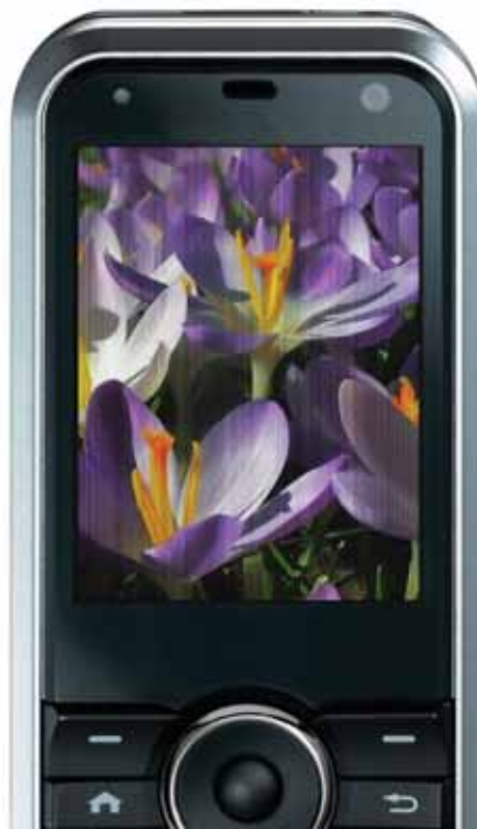
Polysilicon AMOLEDs with conventional compensation (some visible mura)
