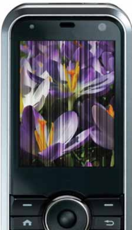
Polysilicon AMOLEDs with no compensation (severe mura)
